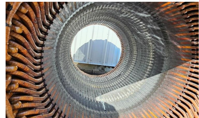
Electric Motor Damaged Stator
